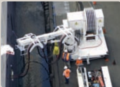
Mobile AMP in the process of delivering shore-to-ship power at Port of Los Angeles.
