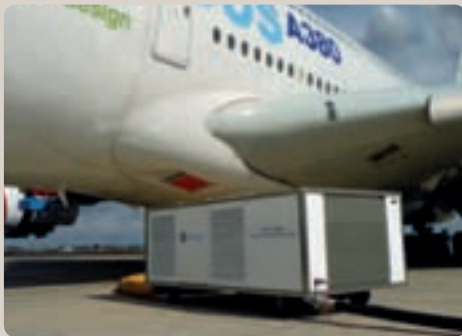
Cavotec's unique PCAir system is able to cool even the largest aircraft such as the A380.
