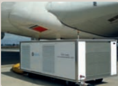
Even in hot climates the PCAir system continues to provide cool compressed air.
