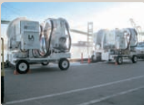
Port of Los Angeles ferry terminal uses mobile AMP for many of their visiting ferries.
