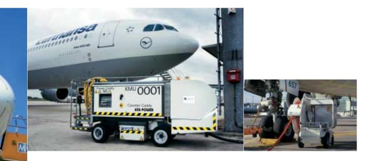
One of our newest innovations is the PCA Caddy. This technology has been specifically designed to supply pre-conditioned air to aircraft without using diesel generators or other pollutants. As it is compact and mobile, the PCA Caddy can be used at different gates without any adaptation to the airport infrastructure.
